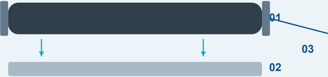
01 Edge and sealed ends / 02 Mounting base / 03 Cable and strain relief
